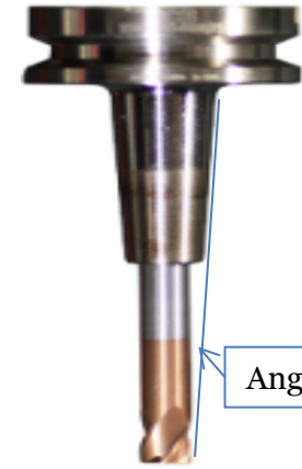
D12R1L65 After machining tool number "P3~P5", Semi-Finishing for deep and small angle
