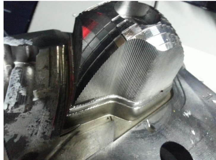
300X200 cutting depth:130 CornerRo.3
