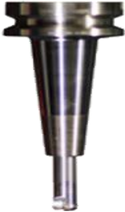
D15R3.5L40 Roughing clearance 0.3 Semi-Finishing(Contour) 0.06
