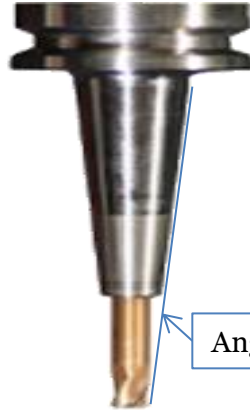
D10R1L40 After using tool number "P3", Rest-Semi-Finishing for machining area with short tool
